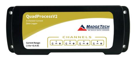
The QuadProcessV2 is an 4-channel, battery powered, low level DC current data logger with a reading rate of up to 4 Hz. It can measure and record 130,944 readings per channel. To maximize memory capacity, users can enable or disable channels. For easy identification, each channel can be named with up to a ten digit title.
