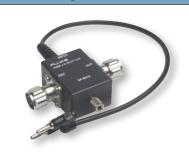
The low current adapter is used to calibrate shunts at currents levels of 2 A or less. It connects together the current source and two shunts for calibration measurements. This adapter mates with N-type connectors to the shunts and a dual banana connection to the source. In this configuration, a certified or reference shunt is connected in series with a shunt that is being calibrated, which in turn are in series with a current source.
