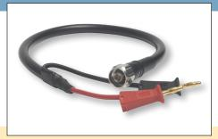
This lead permits connecting the A40B shunt's N-type connectors to instrumentation that uses dual banana plug connection terminals. Using two leads permits connecting the shunt's voltage output to a voltage measuring instrument and also connecting the shunt's current input to a UUT current source rated 20 Å or less.
