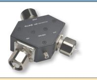
The high current adapter is used when calibrating the A40B shunts at current levels of more than 2 A. It connects together the current source and two shunts for calibration measurements. This adapter uses LC connectors. In this configuration, a certified or reference shunt is connected in series with a shunt that is being calibrated, which in turn are in series with a current source.
