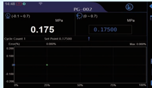
Pressure gauge / transmitter / switch calibration
