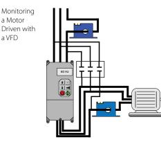
Use the ATR current transducer on the line or load side of the drive and the signal will be accurate in either position.
