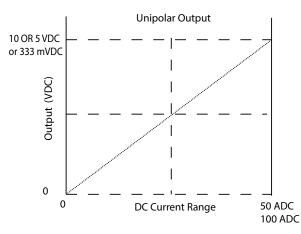
Output remains accurate even as the temperature rises and falls from -20°C to +50°C (-4 to +122 °F) with our patent pending design.
