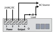
Display shows trip point in amps so 15 A displays 015.
