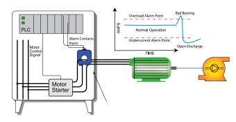
Pumps draw more current when there are mechanical problems like seizing bearings or obstructed impellers, and draw less current when the intake suction is blocked or the discharge is not connected.
