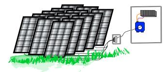
Commercial and industrial ground mounted solar arrays are connected in series to combiner boxes, developing higher voltage and lower current to deliver the same power as with a lower voltage system.
