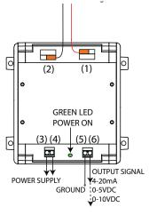
(3) Supply Voltage24U 24 VAC/DC external power supply
