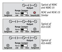
Note: Terminals are #6 screws. DC contacts are polarity sensitive.
