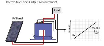
The DT sensor will produce a signal directly proportional to the current produced by the panel or string of panels, with an output to match the controller being used.
