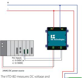
provides a change in output signal polarity when the monitored voltage polarity reverses. Positive on upper right terminal creates a positive output signal; positive on upper left terminal creates a negative output signal.
