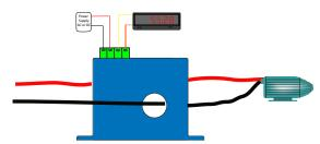
Use a DT sensor over one lead to a DC motor to measure the current used. Over normal readings mean a jam or a bearing failure, and under normal current means a belt or coupling may have broken. The output can also be used to measure time of use to help with maintenance scheduling.
