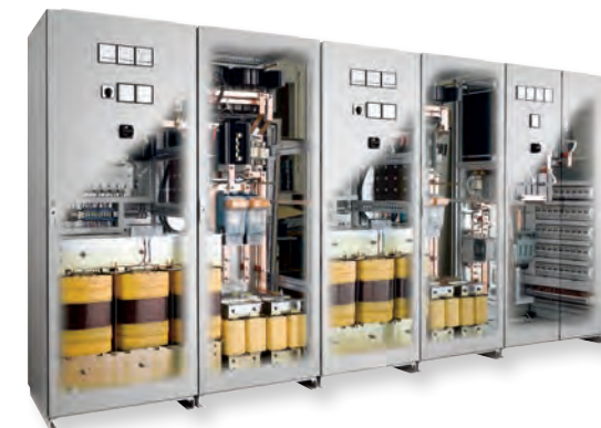
400kW aircraft engine test, 290V DC power supply system, dual 700A configuration for highly inductive load (turbine)
