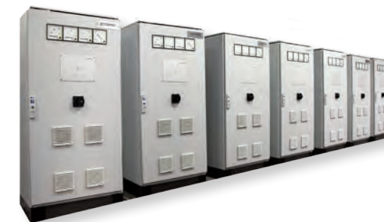
DC power 200kW for the airport, 110 VDC power generation, dual 800 A configuration, full load operation up to +55 °C ambient temperature, protection degree IP42
