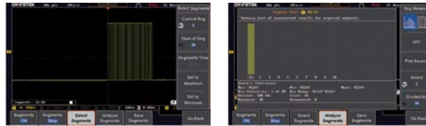
Users Can Select “Analyze Segments” to Conveniently Obtain The Analysis Results.
