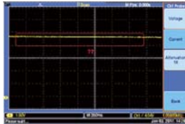
Aliasing due to the insufficient sample rate
