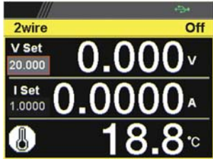
White: Temperature Control on with GTL-205A Connected
