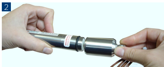
Figure 1 – Removing thermo cover from TCTemp1000 data logger body. Note the right hand is holding the cable gland, and the thermo cover is being removed from the TCTemp1000 data logger body.
