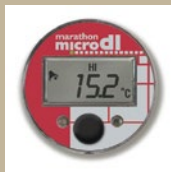
4. HI: 15.2°C shows alarm has occurred and high temperature
