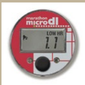
7. LOW HR: 1.1 shows alarm time hours over low threshold
