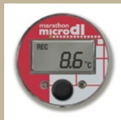
1. REC: 8.6°C shows recording and current temperature
