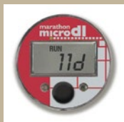
2. RUN: 11 D shows elapsed time in days
