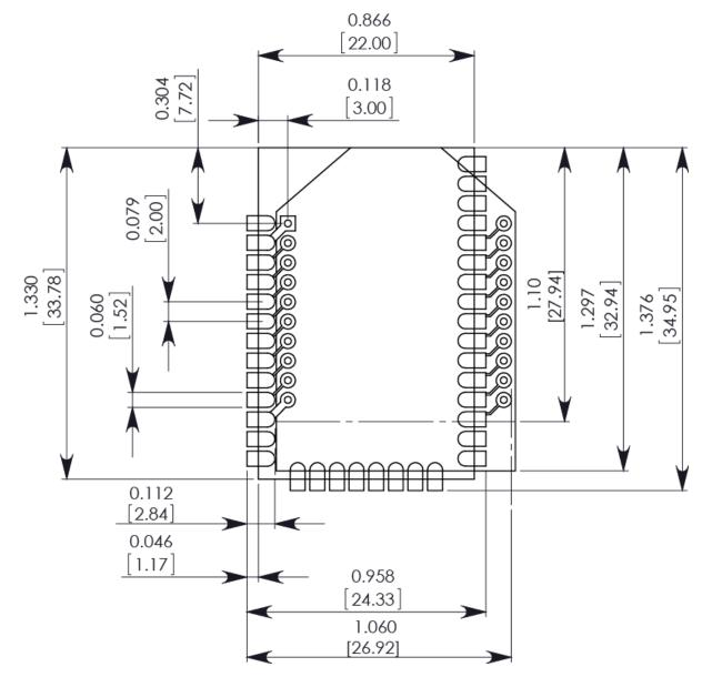
The round holes in the drawing are for the through-hole version, and the semi-oval pads are for the surface mount version. Pin 1 of the through-hole version connects with pin 2 of the surface mount. Use the diagonal traces to connect the pins and the layout will work for both devices.
