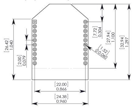
Match the solder footprint to the copper pads. You may need to adjust the footprint depending on the specific needs of assembly and product standards. The underside of the device is mostly coated with solder resist, but we recommend that you leave the copper layer directly below the device open to avoid unintended contacts. Copper or vias must not interfere with the three exposed RF test points on
