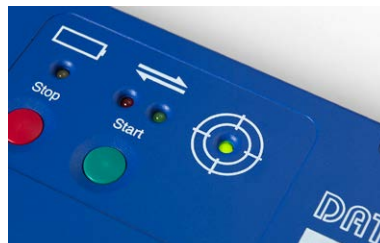
ET3 logger SmartPaq* – “Pass/Fail” indication from logger
