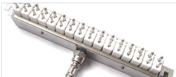
VACQ III external connection box
