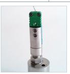
NanoVACQ 1Th with micro-connector and connected type K thermocouple
