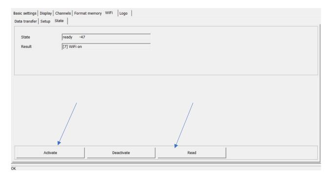
If the "ready" and "WiFi on" indicators for status and result appear, the logger is successfully connected to your WiFi connection and the local server (background process of the application) and the measurement data is sent.
