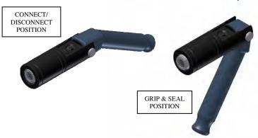
The Jaws JXL Connectors provide a reliable leak-tight connection that grips and seals straight tubing. Simply place the JXL connector onto a tube, activate the mechanical gripping and sealing action, then introduce the test media. For vacuum to 1000 psi applications with air, gas or liquid, Fastest The Jaws JXL Connectors provide secure, leak tight sealing.
