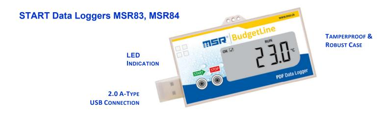
Check the status of the data logger: During recording [RUN] & Stop [STOP] mode, press the START button once to view MIN | MAX | AVERAGE values.
