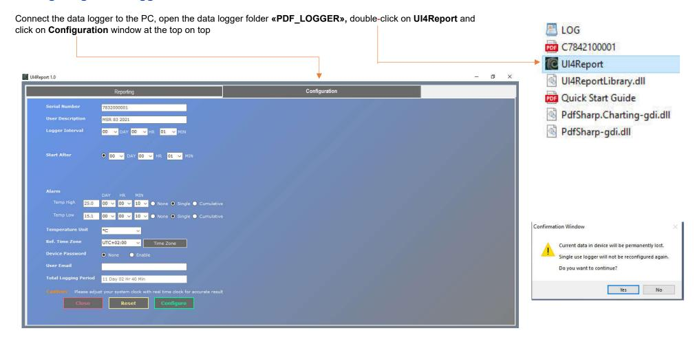
Enter User Description, Logger Interval, Start After (delay start time), Alarm Limit, Alarm Delay Time, Alarm Type, Temperature Unit, Time Zone, Device Password (optional), User Email (optional) and click on **Configure.**
