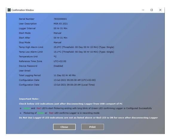
Just after disconnecting the data logger, the green and the red LED will start flickering and then the green LED will be ON for a second indicating the configuration of the logger has completed successfully.
