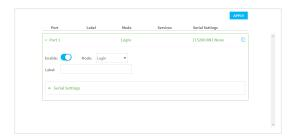
The serial port is enabled by default. To disable, toggle off **Enable**.
