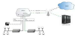
To accomplish this, we will create separate WWAN interfaces that use the same modem but use different APNs, and then use routing roles to forward traffic to the appropriate WWAN interface.
