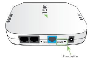
2. Press and hold the **ERASE** button perform a device reset. The **ERASE** button has two modes:
