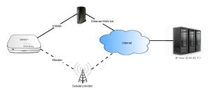
In this example configuration, SureLink is used over for the **WAN** interface to send a probe packet of size **256** bytes to the IP host **43.66.93.111** every **10** seconds. If there are three consecutive failed responses, the EX15 device brings the **WAN** interface down and starts using the **Modem** interface. It continues to regularly test the connection to **WAN**, and when tests on **WAN** succeed, the device falls back to **ETH1**.
