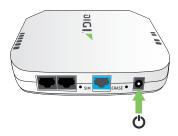
b. Verify that the signal strength indicator on the front of the EX15 shows 2 or more bars, and that the LTE LED on the front of the EX15 shows either green or blue (solid or flashing) for proper operation.
