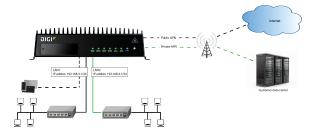
To accomplish this, we will create separate WWAN interfaces that use the same modem but use different APNs, and then use routing roles to forward traffic to the appropriate WWAN interface.
