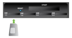
4. After all SIM cards are in place, replace the SIM slot cover.
