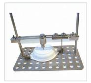
NanoVACQ Deformation with positioning kit for static autoclave
