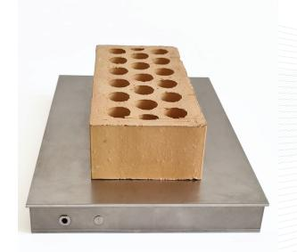
DryBal is a 3 cm high scale which logs mass variations in bricks, tiles or ceramics during drying processes.
