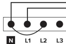
The PowerScout HD Meter uses the Neutral terminal as a voltage reference. For systems without a neutral conductor, connect a wire from the N terminal to ground.
