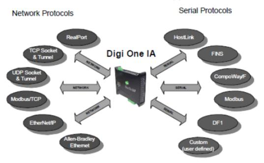
The following table provides a list of serial-port protocols and compatible network protocols. The table also lists which protocols support multi-mastering, a feature that allows multiple masters, each of which may use a different network protocol, to manage a slave simultaneously.
