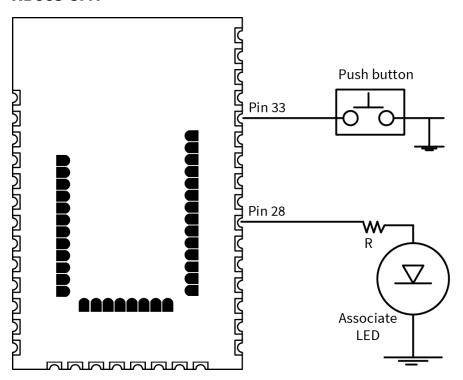
A pushbutton and an LED can be connected to the surface-mount device to support the commissioning pushbutton and associate LED functionalities.
