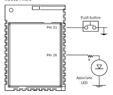
A pushbutton and an LED can be connected to the Micro device to support the commissioning pushbutton and associate LED functionalities.
