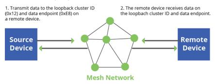
4. Source receives loopback transmission and sends received packet out the serial port.
