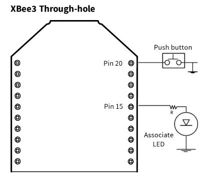
A pushbutton and an LED can be connected to the through-hole-mount device to support the commissioning pushbutton and associate LED functionalities.
