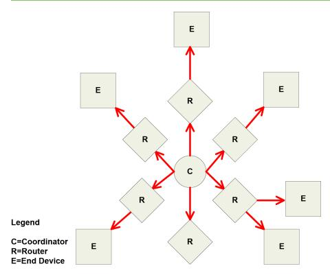
Each node that transmits the broadcast also creates an entry in a local broadcast transmission table. This entry to keeps track of each received broadcast packet to ensure the packets are not transmitted endlessly. Each entry persists for 8 seconds, and the broadcast transmission table holds 8 entries, effectively limiting network broadcast transmissions to once per second.
