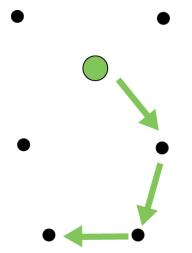
A remote device sends an RF data packet to the data collector. This is prefaced by a route record transmission to the data collector.
