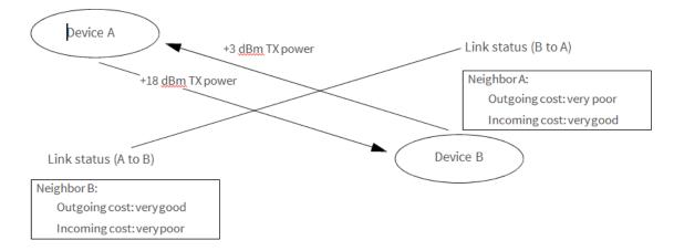
This mechanism enables devices A and B to recognize that the link is not reliable in both directions and select a different neighbor when establishing routes. Such links are called asymmetric links, meaning the link quality is not similar in both directions.
