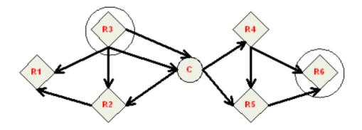
When the destination node receives a route request, it compares the 'path cost' field against previously received route request commands. If the path cost stored in the route request is better than any previously received, the destination node transmits a route reply packet to the node that originated the route request. Intermediate nodes receive and forward the route reply packet to the source node (the node that originated route request).
