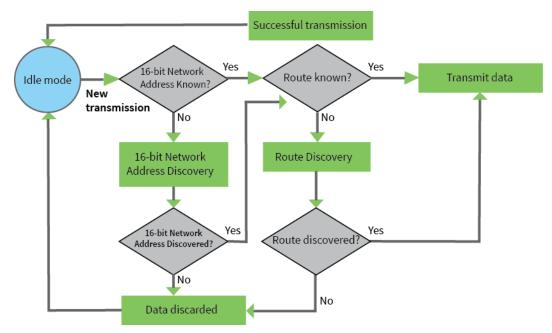
Transmit mode is the mode in which the device is transmitting data. This typically happens when data is received from the serial port.
