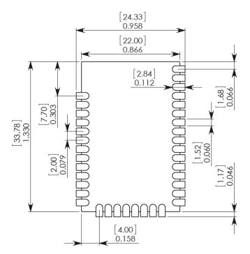
Match the solder footprint to the copper pads, but may need to be adjusted depending on the specific needs of assembly and product standards. Recommended stencil thickness is 0.15mm/0.005". Place the component last and set the placement speed to the slowest setting.
