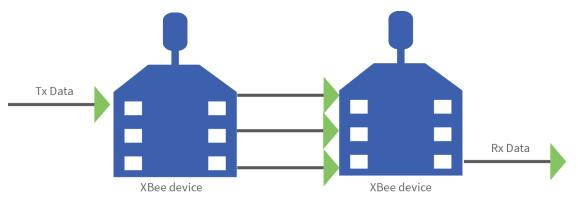
The transmit frame can include up to 255 bytes of data broken up into multiple transmissions and reassembled on the receiving side. If one or more of the fragmented messages are not received by the receiving device, it drops the entire message, and the sender indicates a transmission failure in the Tx Status API frame.
