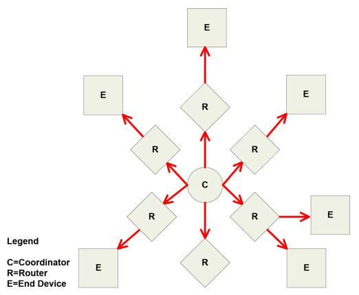
Each node that transmits the broadcast also creates an entry in a local broadcast transmission table. This entry to keeps track of each received broadcast packet to ensure the packets are not transmitted endlessly. Each entry persists for 8 seconds, and the broadcast transmission table holds 8 entries.
