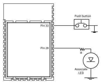
A pushbutton and an LED can be connected to XBee/XBee-PRO ZigBee RF Module pins 33 and 28 (SMT), or pins 20 and 15 (TH) respectively to support the commissioning pushbutton and associate LED functionalities.
