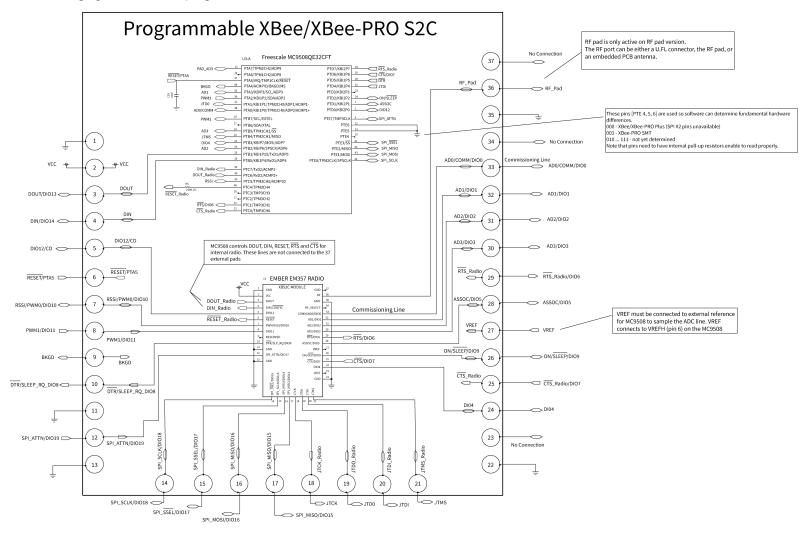
XBee/XBee-PRO® S2C ZigBee® RF Module
