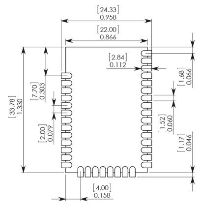
Match the solder footprint to the copper pads, but you may need to adjust it depending on the specific needs of assembly and product standards. We recommend a stencil thickness of 0.15 mm (0.005 in). Place the component last and set the placement speed to the slowest setting.
