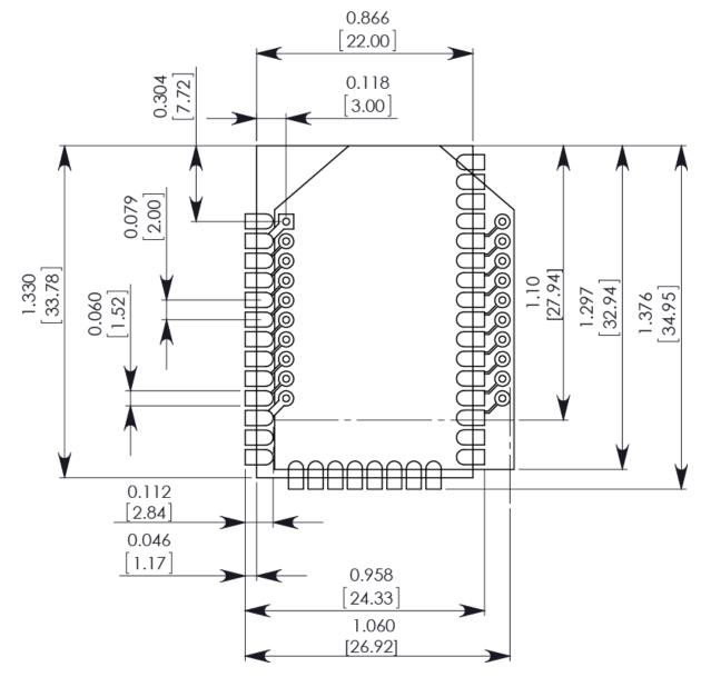
The round holes in the diagram are for the TH design, and the semi-oval pads are for the SMT design. Pin 1 of the TH design is lined up with pad 1 of the SMT design, but the pins are actually offset by one pad; see Pin mapping. By using diagonal traces to connect the appropriate pins, the layout will work for both devices.
