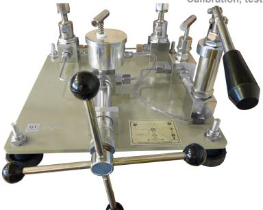
**HIGHLIGHTS Precision screw pump** Rotatable process connections (2 shots) Low maintenance
