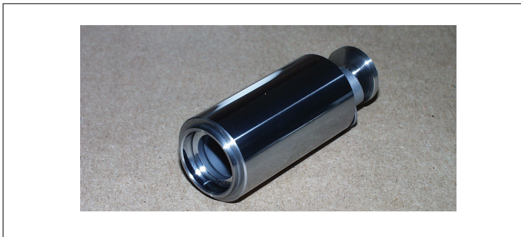
Figure 5-6. Low Range Piston and Cylinder Showing O-Ring Groove
