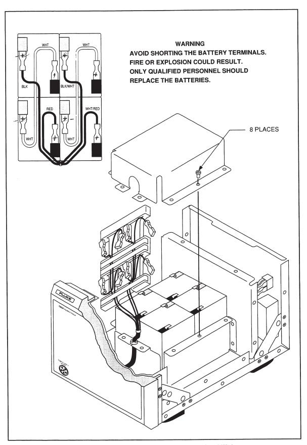
Figure 5-3. Accessing the Battery and Battery Lead Wiring
