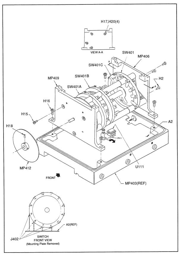
Figure 6-1. Sensor Unit Final Assembly (cont)
