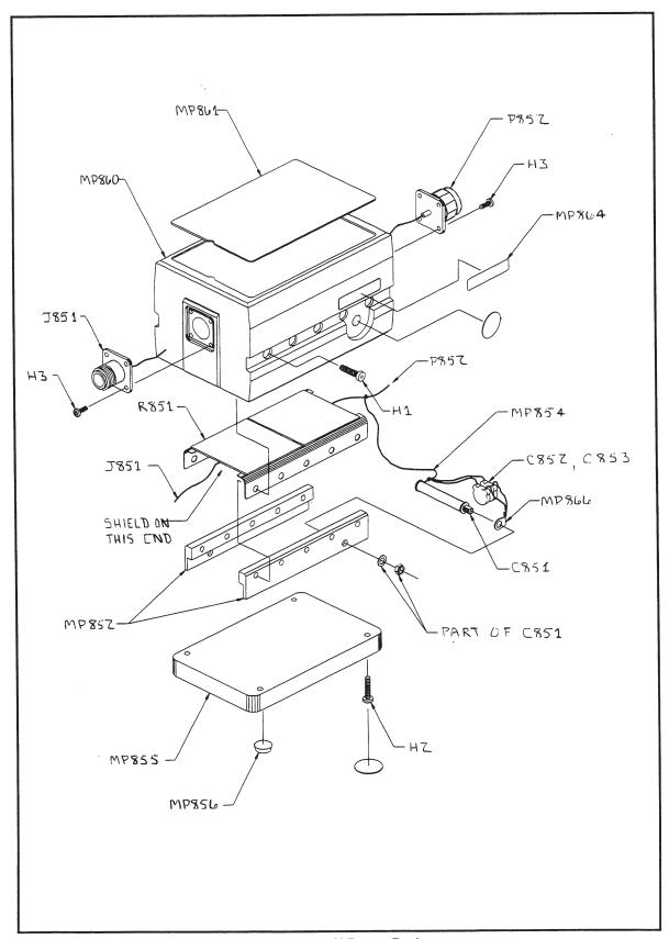
Figure 6-6. 1000V Range Resistor
