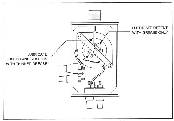
Figure 5-10. Transfer Switch Lubrication Points
