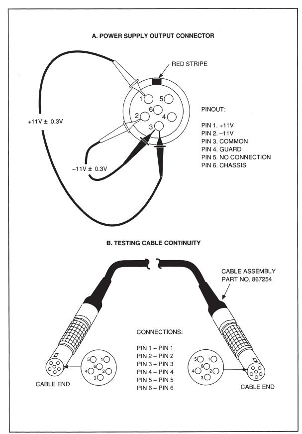
Figure 5-2. Power Pack Cable and Output Voltage
