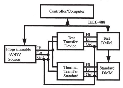
Figure 6. AV/DV Tranfer System Block Diagram
