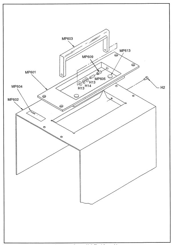
Figure 6-1. Sensor Unit Final Assembly
