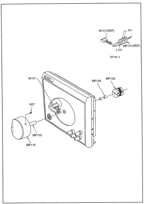
Figure 6-1. Sensor Unit Final Assembly (cont)
