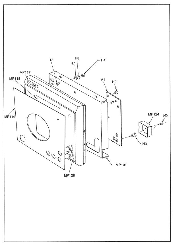
Figure 6-1. Sensor Unit Final Assembly (cont)
