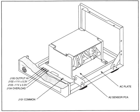
Figure 5-7. AC Plate Voltage Test Points
