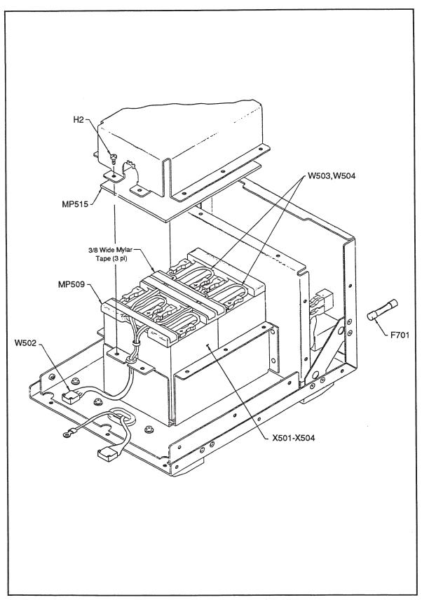
Figure 6-4. Power Pack Final Assembly (cont)
