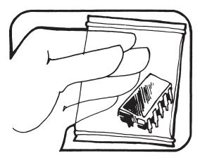
5. USE ANTI-STATIC CONTAINERS FOR HANDLING AND TRANSPORT
