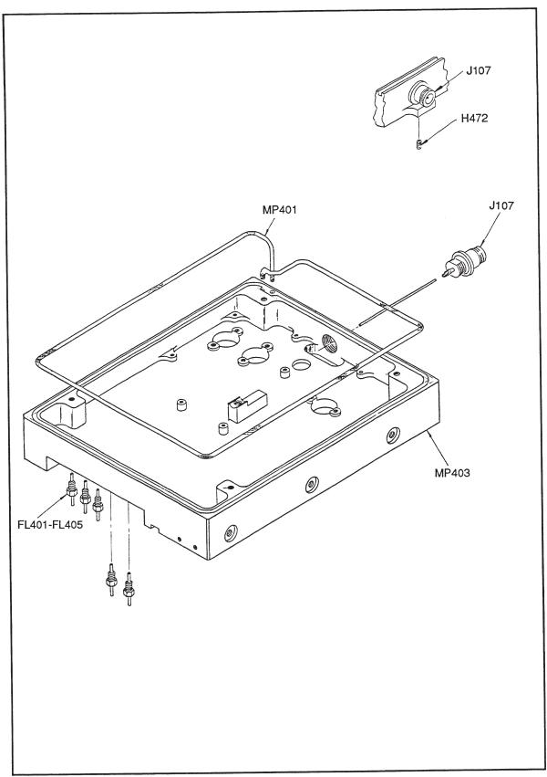
Figure 6-1. Sensor Unit Final Assembly (cont)
