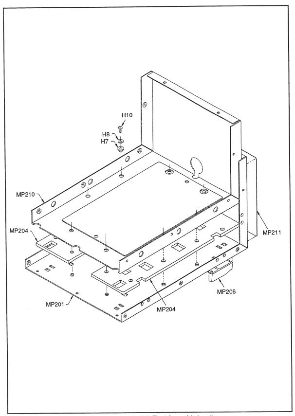
Figure 6-1. Sensor Unit Final Assembly (cont)
