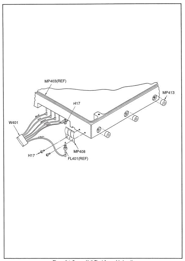
Figure 6-1. Sensor Unit Final Assembly (cont)
