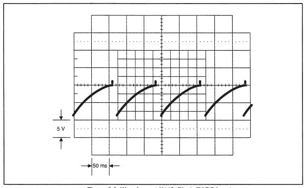
Figure 5-9. Waveform at U112, Pin 1, 5V DC Input
