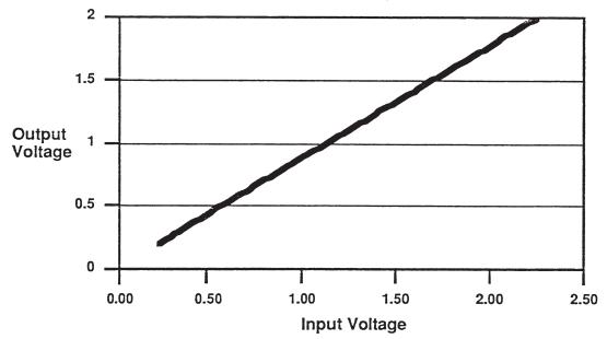
Figure 2. Linearity: 2 V Range, 0.22 to 2.2 Volts
