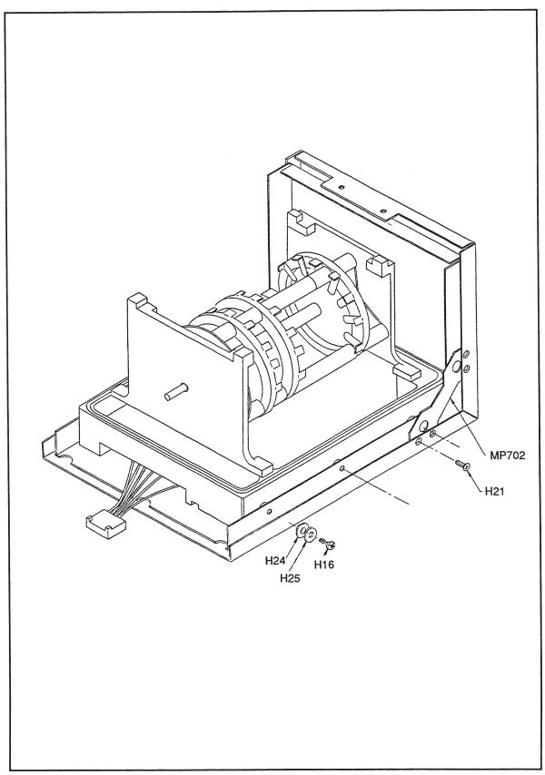
Figure 6-1. Sensor Unit Final Assembly (cont)
