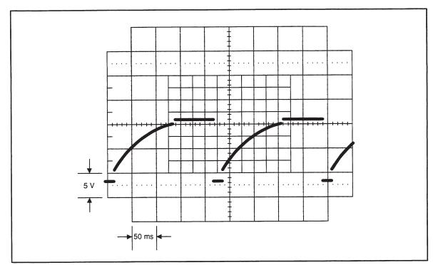
Figure 5-8. Waveform at U112, Pin 1, 3.5V DC Input
