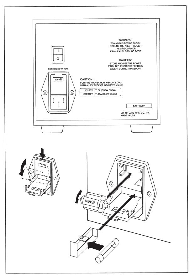
Figure 2-2. Fuse Rating Label and Fuse Location
