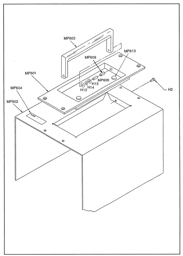
Figure 6-4. Power Pack Final Assembly
