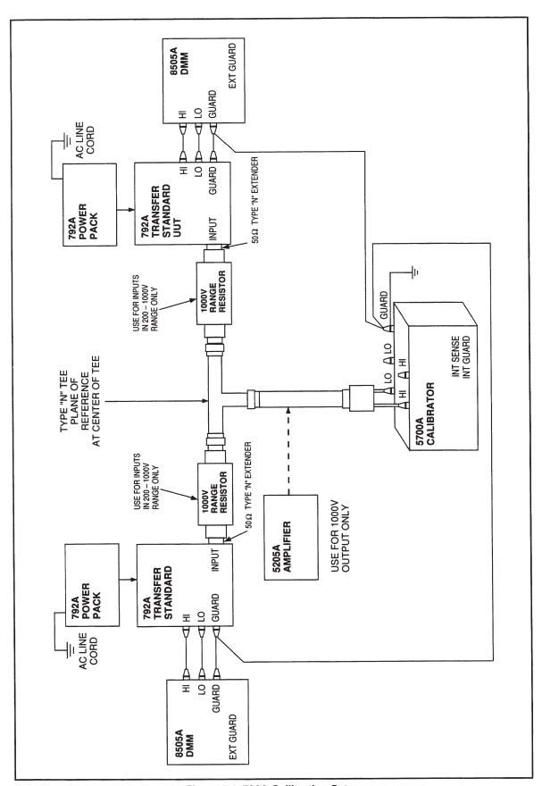
Figure 5-1. 792A Calibration Setup
