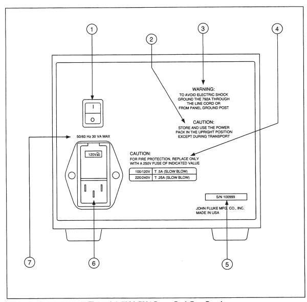
Figure 3-4. 792A-7001 Power Pack Rear Panel
