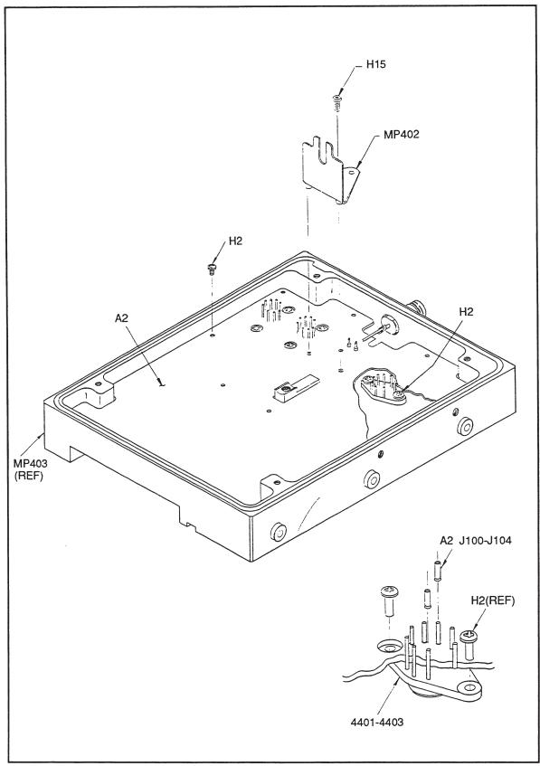
Figure 6-1. Sensor Unit Final Assembly (cont)
