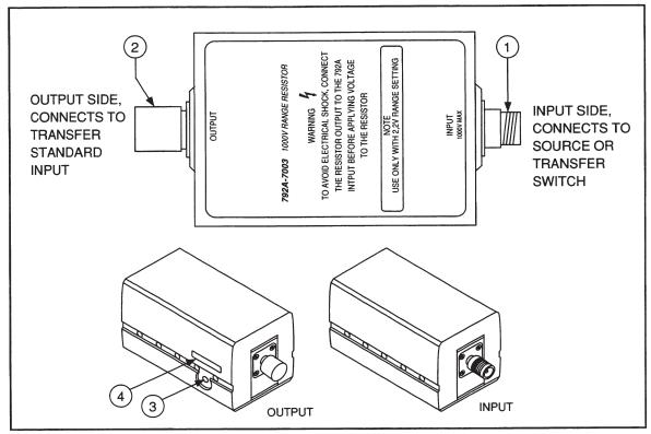
Figure 3-5. 792A-7002 1000V Range Resistor
