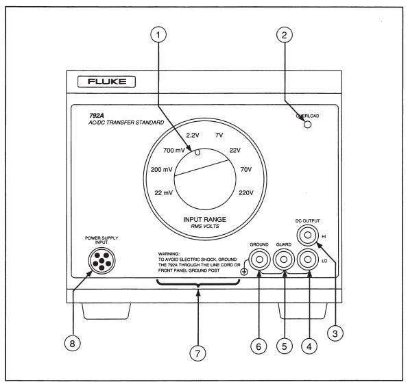
Figure 3-1. 792A AC/DC Transfer Standard Front Panel
