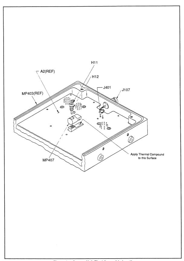
Figure 6-1. Sensor Unit Final Assembly (cont)
