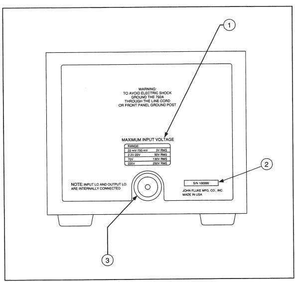
Figure 3-2. 792A AC/DC Transfer Standard Rear Panel
