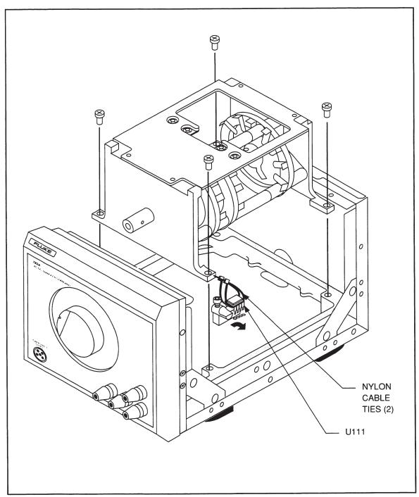
Figure 5-4. Replacing U111
