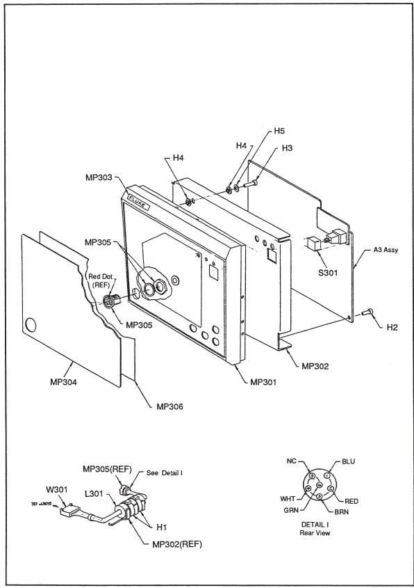
Figure 6-4. Power Pack Final Assembly (cont)
