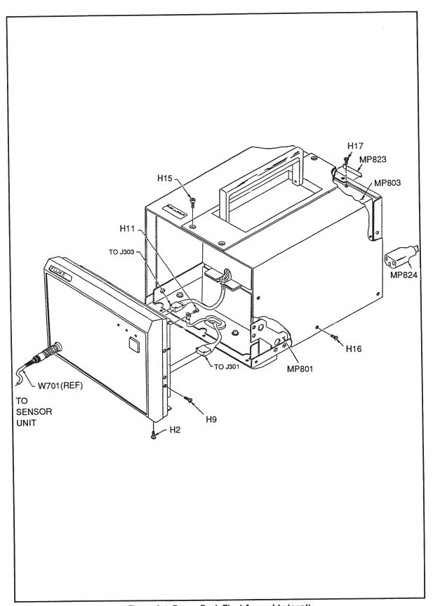
Figure 6-4. Power Pack Final Assembly (cont)
