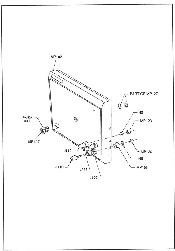
Figure 6-1. Sensor Unit Final Assembly (cont)
