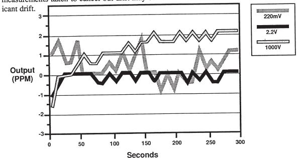
Figure 4. 792A Output Settling: 220 mV, 2.2 V & 1000 V Ranges
