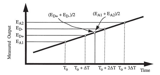
Figure 1. Thermal Drift Compensation
