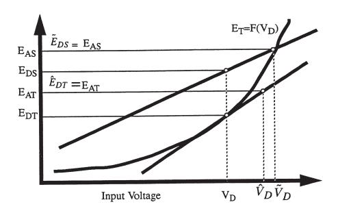
Figure 7. Linearization of the Test Device
