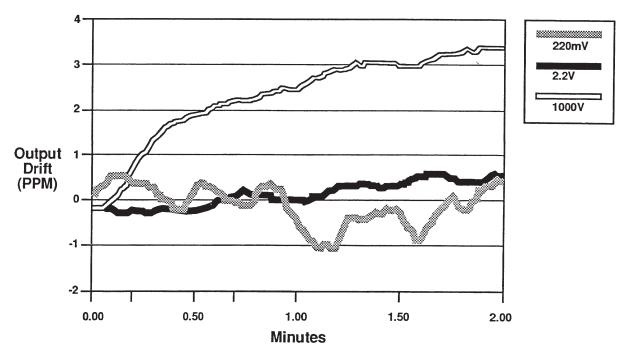
Figure 5. 792A Output Drift: 220 mV, 2.2 V & 1000 V Ranges
