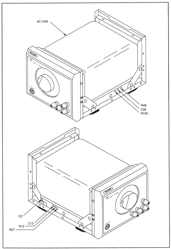
Figure 5-5. Location of Adjustments on the AC Plate
