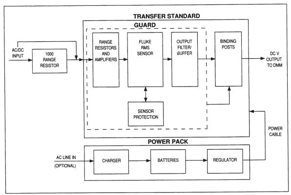
Figure 4-1. 792A Block Diagram
