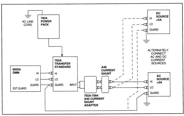
Using the 792A-7004 A40 Current Shunt Adapter
