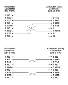
Figure 8 Serial Communications Cable Wiiring
