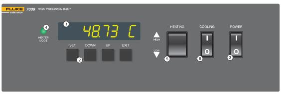
Figure 2 Front Controller Panel
