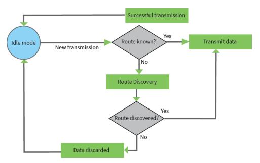
When DigiMesh data is transmitted from one node to another, the destination node transmits a network-level acknowledgment back across the established route to the source node. This acknowledgment packet indicates to the source node that the destination node received the data packet. If the source node does not receive a network acknowledgment, it retransmits the data. For more information, see <u>Data transmission and routing</u>.
