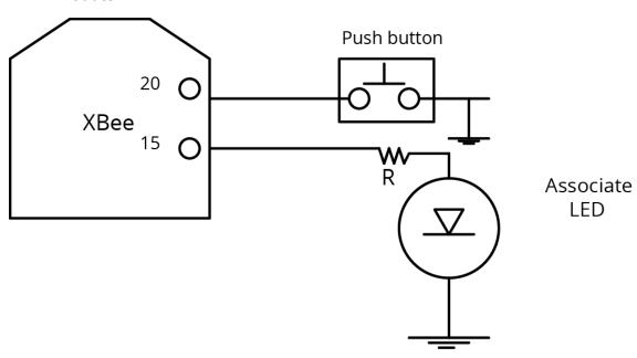
Connect a pushbutton and an LED to XBee-PRO 900HP RF Module pins 20 and 15 respectively to support the commissioning pushbutton and associate LED functionalities.
