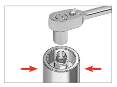
3. Holding the smooth metal end of the stopper, use a 7/16" wrench or socket to tighten the body into the stopper.
