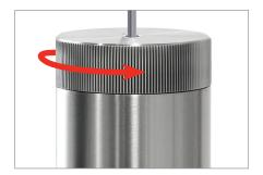
7. Insert the data logger and stopper assembly back into the thermal barrier and screw the endcap of the thermal barrier until the O-Ring is no longer visible.
