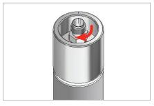
**2.** Screw the Fitting Body into the end of the stopper assembly (finger-tight).
