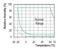
Long term exposure to humidity levels outside of the 'normal' range may temporarily offset RH measurements (±3%RH after 60 hours). Once returned to less extreme conditions the device will slowly return towards calibration state.
