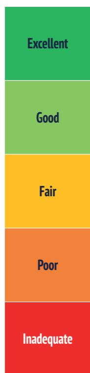
The colour of the status ring shows the current IAQ level. If the IAQ is Poor or Inadequate the status ring will turn red and the sounder, if activated, will beep to alert those nearby. If you have configured email or SMS notifications on the Cloud these will automatically be sent to your selected recipients.
