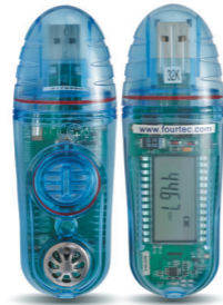
Internal Temperature & Humidity LITE5032L-RH
