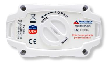
Remove the old battery and discard to an appropriate recycling system. With a new, fresh, CR2450 battery, position the battery with the "+" symbol up towards you. Deposit the battery into the LynxPro. You may find some reluctance due to a tight fit. The battery should be snug but not require significant force. Once inserted/centered, apply the battery plug and rotate 45 degrees to lock the plug into place.
