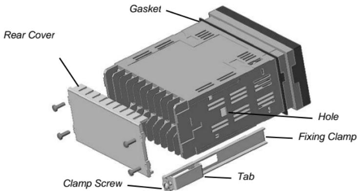
**Figure 2: Mounting the Monitor**
