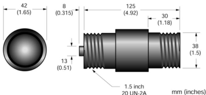
**Figure 30: Dimensions for the GPR Head**
