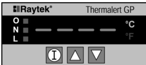
**Figure 10: The Control Panel Start-up Screen**
