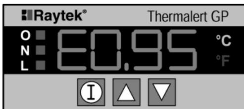
Figure 12: Emissivity Display
