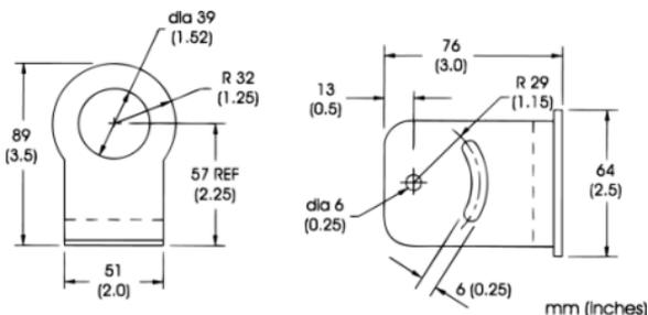
**Figure 34: Fixed Mounting Bracket**
