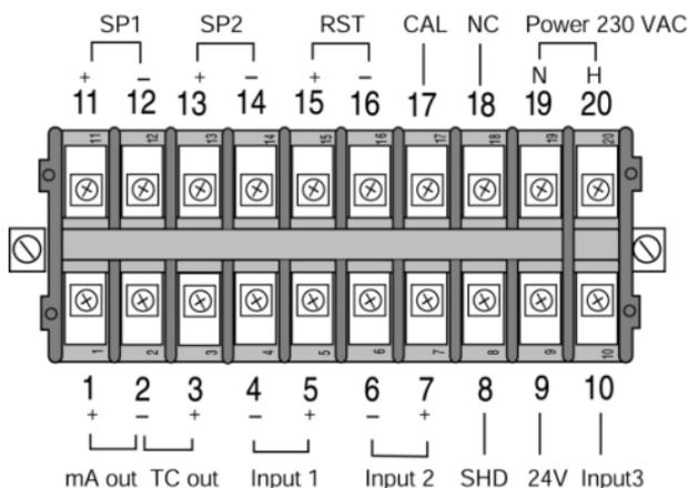
**Figure 6: Terminal Block Layout**
