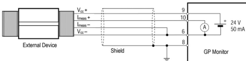
**Figure 7: Installation 4 – 20 mA (4 Wires)**
