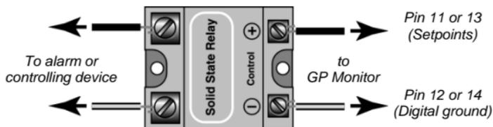
**Figure 9: Relay Accessory Wiring**
