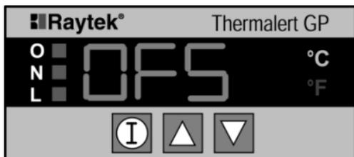
Figure 24: Offset Indicator Display
