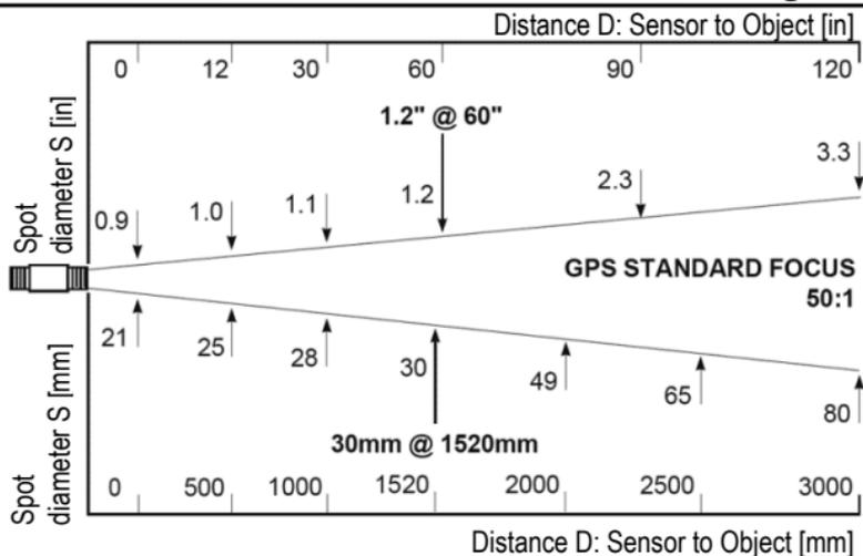
Figure 43: GPS Standard Focus Optics
