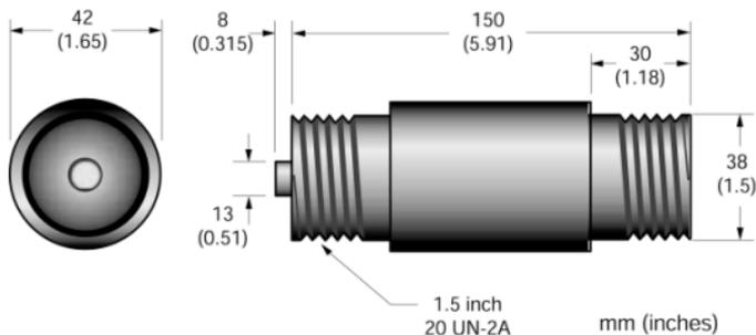
**Figure 31: Dimensions for the GPS Head**
