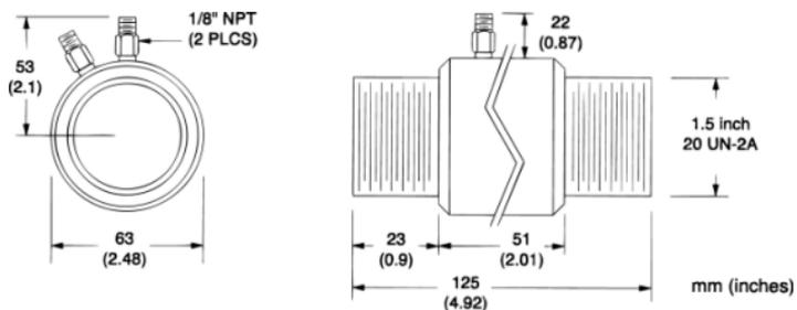
**Figure 35: GPR Head with Air/Water-cooled Housing**
