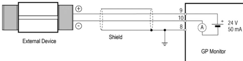
**Figure 8: Installation 4 – 20 mA (2 Wires)**
