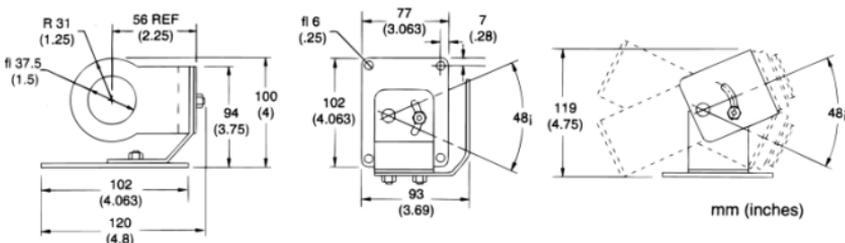
Figure 37: Adjustable Mounting Bracket
