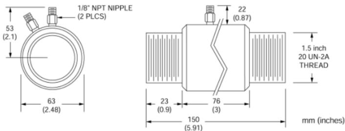
**Figure 36: GPS Head with Air/Water-cooled Housing**
