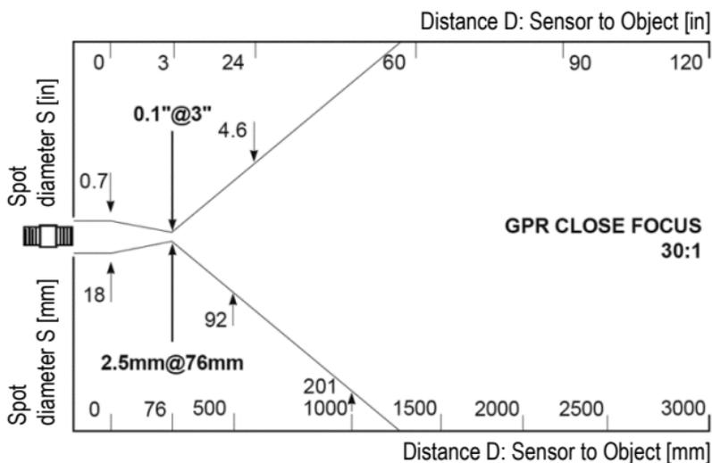
Figure 42: GPR Close Focus Optics
