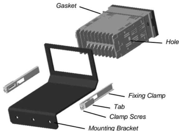
**Figure 3: Mounting Bracket Accessory Installation**
