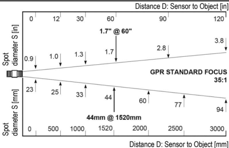
Figure 41: GPR Standard Focus Optics
