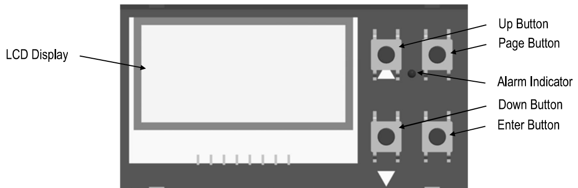
Figure 33: Control Panel for the Comm Box (DIN)
