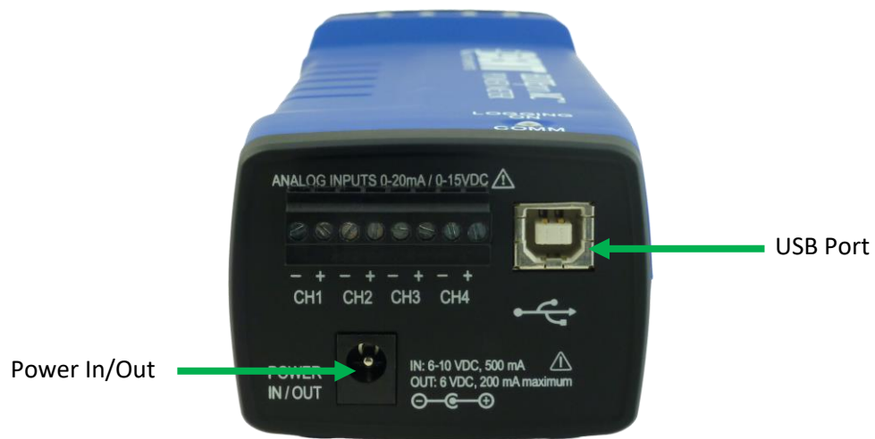
Power End Panel Connections
