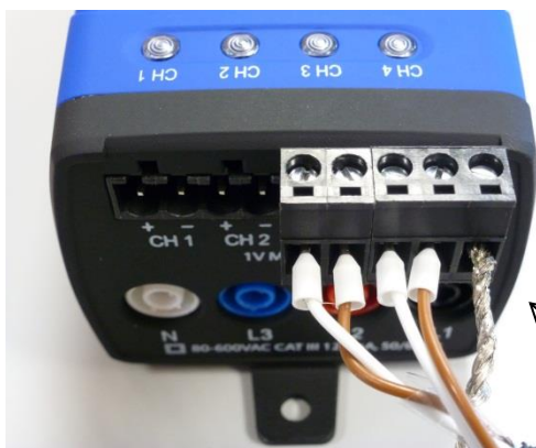
Connecting RōCoil CTs to an ELITEpro XC
