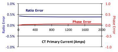
CT testing performed with 16"RoCoil. Conductor used filled 90% of RoCoil window.
