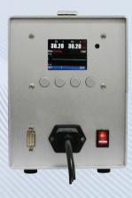
The BL671 is a small size blackbody calibration source utilizing a digital indicating temperature ambient 30°C to 50°C (86F to 122F). A 70x70 mm size ridged plate is heated or cooled with an internal solid state thermoelectric heat pump. It has a builtin digital temperature controller to provide accurate, stable temperature as well as to provide readout.
