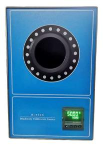
With isothermal cavity, the BL672S is a portable blackbody calibration source utilizing a digital indicating temperature ambient 20°C to 50°C (68F to 122F). The 80 mm diameter end closed tube is heated or cooled with an internal solid state thermoelectric heat pump. It has a built-in digital temperature controller to provide accurate, stable temperature as well as to provide readout.
