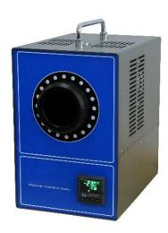
The BL673 is a portable blackbody calibration source utilizing a digital indicating temperature from -20°C to 125°C. A precision platinum RTD temperature sensor is embedded in the blackbody emitter, providing high accuracy and repeatability.
