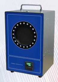
The BL675A is a portable blackbody calibration source utilizing a digital indicating temperature ambient 50°C to 500°C. A precision platinum RTD temperature sensor is embedded in the blackbody emitter, providing high accuracy and repeatability. The temperature controller uses the industry standard PID algorithms to control the emitter temperature to within 0.1% of the set points.
