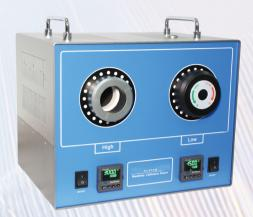
The BL675D Dual Cavity Blackbody Calibration Source is easy to use, and makes calibration of infrared pyrometers with multiple temperature ranges faster than ever before by combining a hot and cold side in one unit.
