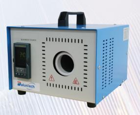
The BL676 is a portable blackbody calibration source utilizing a digital indicating temperature ambient  $35^{\circ}$ C to  $500^{\circ}$ C. A precision platinum RTD temperature sensor is embedded in the blackbody emitter, providing high accuracy and repeatability. The temperature controller uses the industry standard PID algorithms to control the emitter temperature to within 0.1°C of the set points.
