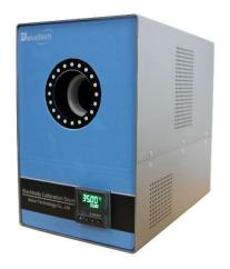
The BL676 is a portable blackbody calibration source utilizing a digital indicating temperature ambient  $35^{\circ}$ C to  $500^{\circ}$ C. A precision platinum RTD temperature sensor is embedded in the blackbody emitter, providing high accuracy and repeatability. The temperature controller uses the industry standard PID algorithms to control the emitter temperature to within  $0.1^{\circ}$ C of the set points.
