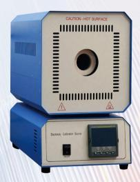
The BL678A is a benchtop blackbody calibration source utilizing a digital indicating temperature ambient 100°C to 1200°C. A precision thermocouple N temperature sensor is embedded in the blackbody emitter, providing high accuracy and repeatability. The temperature controller uses the industry standard PID algorithms to control the emitter temperature to within 0.1°C of the set points.
