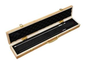
The BL619 Standard thermocouple are measurement standards for temperature, featuring a simple structure, high accuracy, excellent physical and chemical performance, strong oxidation resistance at high temperatures, and excellent stability and reproducibility of thermoelectric potential.
