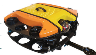
S-ROV with optional gripper
