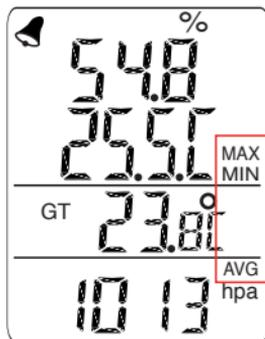
**Note:** When the meter is MAX/MIN/AVG function, the **HOLD** and **MODE** buttons are disabled.
